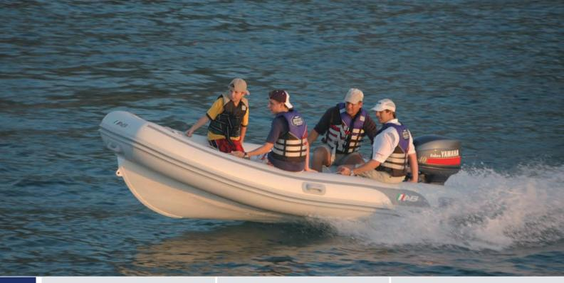
ے 2 Overal Length : 14'/ 4.27m Number of Chambers : 4 Maximum HP : 50hp / 37.3kw **Overal Beam Person Capacity** : 8 : 6'7"/ 2.00m Shaft Length : 20" / 50.8cm Inside Length : 10′10″/3.30m : 246lb/112kg Weight RDC Design Category : C Inside Beam : 3'3"/ 0.99m Weight with Bow Locker: 264lb/120kg Tube Diameter : 19"/ 0.48m Recommended HP : 40hp/29.8kw
