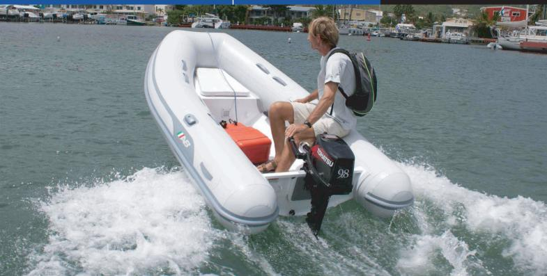
**Overal Length** : 9'6"/ 2.90m **Number of Chambers** Maximum HP : 15hp / 11.2kw **Overal Beam Person Capacity** : 5 : 5'6"/ 1.68m Shaft Length : 15" / 38.1cm Inside Length Weight : 95lb / 43kg : 6'11"/ 2.11m RDC Design Category : C Inside Beam Weight with Bow Locker: 108lb/49kg : 2'6"/ 0.76m
