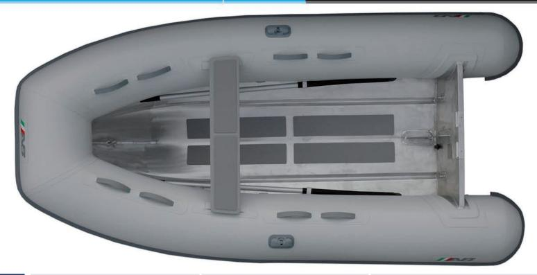
**Overal Length** Shaft Length : 10'/ 3.05m Number of Chambers : 3 : 15" / 38.1cm **Overal Beam Person Capacity** : 5'6"/ 1.68m RDC Design Category : C Weight Inside Length : 7'2"/ 2.18m : 95lb / 43kg Inside Beam : 2'8"/ 0.81m Recommended HP : 8hp / 6.0kw
