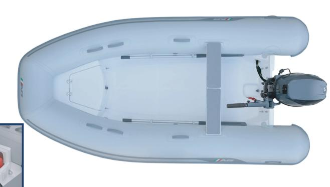
ے 2 **Overal Length** : 12′/3.66m Number of Chambers : 3 + 1Shaft Length Option 1: 15"/38.1cm Shaft Length Option 2:20"/50.8cm **Overal Beam Person Capacity** : 6 6′/ 1.82m RDC Design Category: C Inside Length : 8'9"/ 2.67m Weight : 202lb / 92kg Recommended HP Inside Beam : 2'9"/ 0.84m : 20hp / 14.9kw **Tube Diameter** Maximum HP : 18"/ 0.46m : 30hp / 22.4kw
