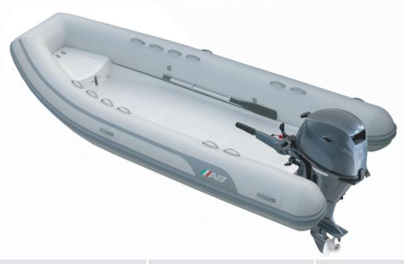
**Overal Length** : 15'/4.57m Number of Chambers : 5 Shaft Length **Person Capacity** RDC Design Category : C **Overal Beam** : 11 : 6'6"/1.99m Inside Length : 11'6"/3.50m Weight : 484lb / 220kg Recommended HP Inside Beam : 3'2"/ 0.97m : 60hp / 44.8kw
