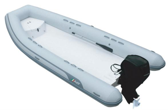
Overal Length : 17′/ 5.18m Number of Chambers : 5 Shaft Length : 20" / 50.8cm **Overal Beam Person Capacity** : 15 RDC Design Category : C : 8'1"/ 2.46m Inside Length : 13'1"/ 4.00m Weight : 772lb / 350kg Inside Beam Recommended HP : 75hp / 56kw
