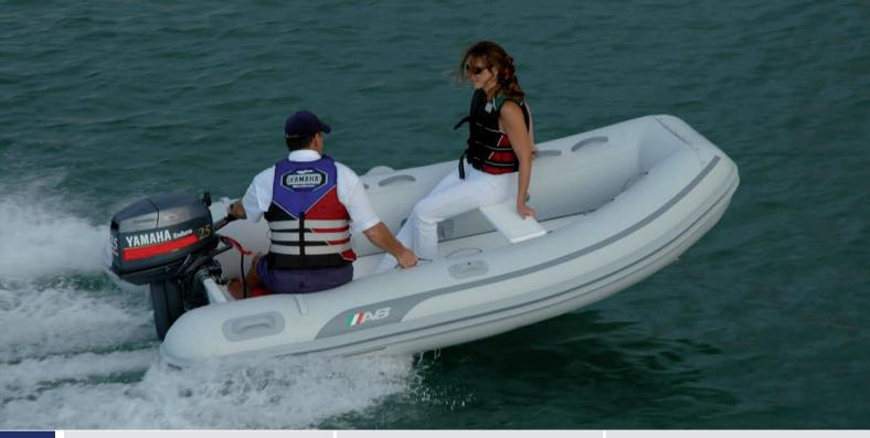
S ட 2 Overal Length : 10'6"/3.19m Number of Chambers : 3 Shaft Length : 15" / 38.1cm : 5'6"/ 1.68m **Person Capacity Overal Beam** : 5 RDC Design Category : C Weight Inside Length : 7'6"/ 2.30m : 117lb / 53kg Inside Beam Recommended HP : 2'8"/ 0.81m : 10hp / 7.5kw
