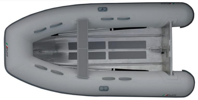
**Overal Length** Shaft Length : 10'/ 3.05m Number of Chambers : 3 : 15" / 38.1cm **Overal Beam Person Capacity** : 5'6"/ 1.68m RDC Design Category : C Weight Inside Length : 7'2"/ 2.18m : 95lb / 43kg Inside Beam : 2'8"/ 0.81m Recommended HP : 8hp / 6.0kw Maximum HP Tube Diameter : 17"/ 0.43m : 9.9hp / 7.4kw
