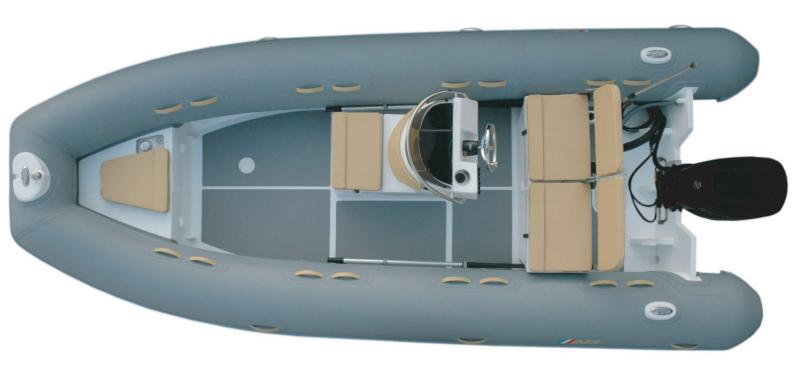
Overal Length : 18′/ 5.49m Number of Chambers : 5 Shaft Length : 25" / 63.5cm **Overal Beam Person Capacity** : 12 Gas Built in Tank : 32 Gal / 120 L : 7' 10"/ 2.40m RDC Design Category : C : 895lb / 406kg Inside Length : 14′8″/4.47m Weight
