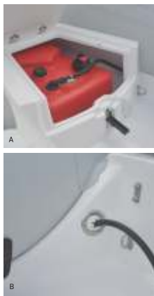
FIGURE A | BOW LOCKER / SEAT TO FIT PORTABLE FUEL TANK (9 TO 12)
