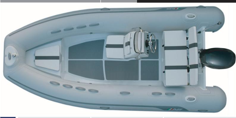
**Overal Length** : 15'/ 4.57m Number of Chambers : 5 **Person Capacity Overal Beam** : 6'9"/ 2.06m : 11'8"/3.55m Inside Length Weight : 467lb / 212kg Inside Beam : 3'4"/1.03m Recommended HP : 50hp/37.3kw **Tube Diameter** : 19"/ 0.48m Maximum HP : 60hp / 44.8kw
