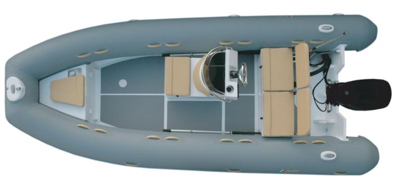
Overal Length : 18′/ 5.49m Number of Chambers : 5 Shaft Length **Overal Beam Person Capacity** : 12 Gas Built in Tank : 7' 10"/ 2.40m RDC Design Category : C Inside Length : 895lb / 406kg : 14′8″/4.47m Weight Inside Beam Recommended HP : 4'3"/ 1.30m : 90hp / 67.1kw
