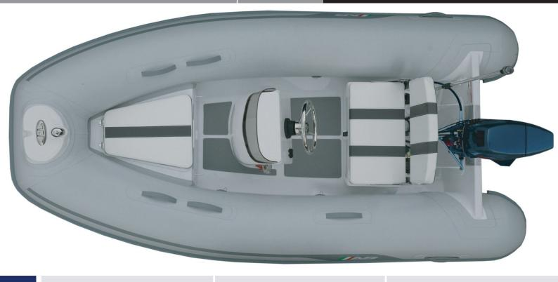
Overal Length : 9'6"/2.90m Number of Chambers : 3 **Person Capacity** : 5 **Overal Beam** : 5′6″/ 1.68m Inside Length Weight : 236lb / 107kg : 6′11″/2.11m Inside Beam : 2'6"/ 0.76m Recommended HP : 10hp / 7.5kw Maximum HP **Tube Diameter** : 17"/ 0.43m : 20hp / 14.9kw
