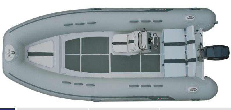
**Overal Length** : 16'/ 4.88m Number of Chambers : 5 Shaft Length **Person Capacity** : 10 RDC Design Category : C **Overal Beam** : 7′/ 2.14m Inside Length : 12'8"/3.85m Weight : 531lb / 241kg Inside Beam : 3'6"/1.08m Recommended HP : 50hp / 37.3kw
