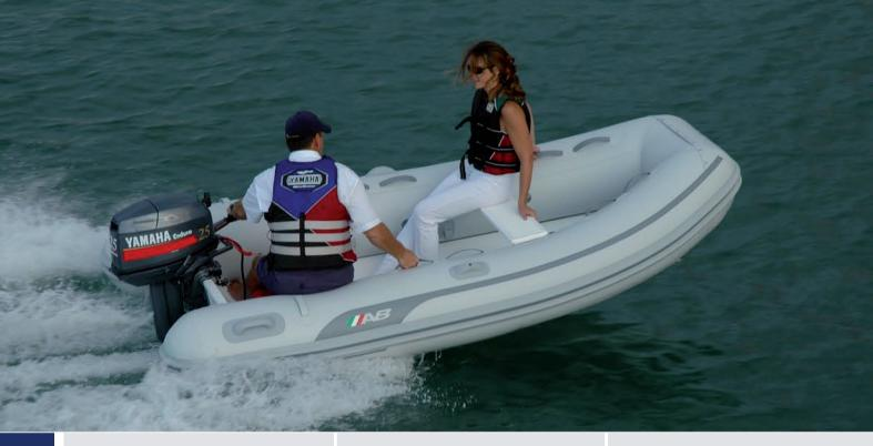
ے S **Overal Length** 10'6"/3.19m Number of Chambers : 3 Maximum HP : 20hp / 14.9kw **Overal Beam Person Capacity** : 5 : 5'6"/ 1.68m Shaft Length : 15" / 38.1cm Inside Length Weight : 117lb / 53kg : 7'6"/ 2.30m RDC Design Category : C Inside Beam : 2'8"/ 0.81m Weight with Bow Locker: 130lb/59kg Tube Diameter : 17"/ 0.43m Recommended HP : 10hp / 7.5kw
