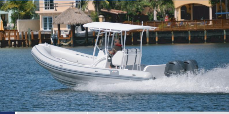
Overall Length : 27′ 4"/ 8.33m Number of Chambers Shaft Length : 30" / 76.2cm Gas Built in Tank Overall Beam : 10′1"/3.07m Person Capacity : 189 Gal / 715 L Inside Length : 22′11"/ 6.99m Weight : 2853lb / 1297kg Water Built in Tank : 12 Gal / 45 L : 6'4"/ 1.93m Recommended HP Inside Beam : 250hp / 186.5kw RDC Design Category: B
