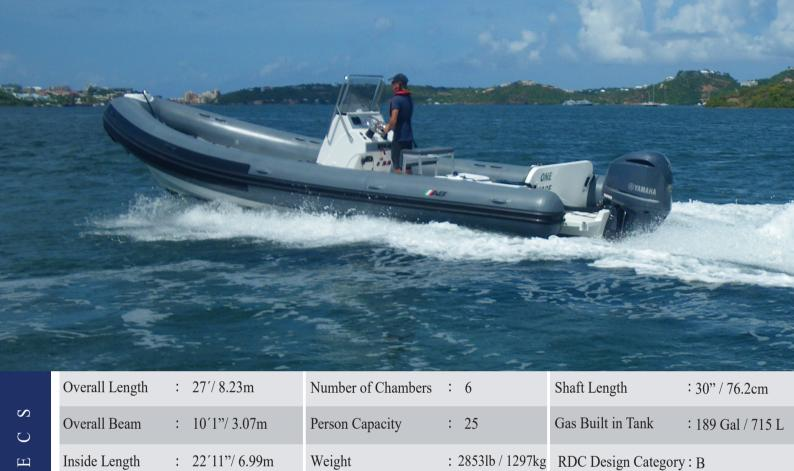
Professional Grade Hand Laid Fiberglass Deep "V" Hull Stringer System Laminated into Hull Diamond Shape Non-skid Deck Integrated Marine Grade Aluminum Fuel Tank Plastic External Transom Plate Aluminum Internal Transom Plate 2 Front & 8 Side Orca (CSM) Fabric Handles on Tubes Life Line Around Tube Non - Skid (CSM) Coated Fabric on Tube's Surface Pressure Relief Valves
