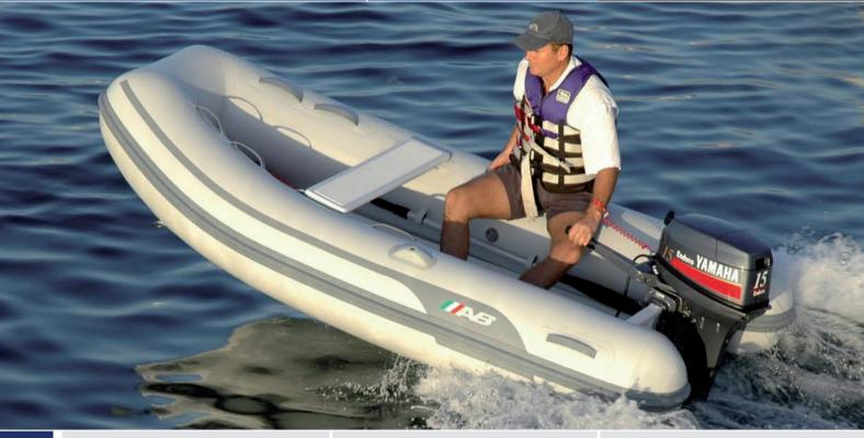
ے S Overal Length : 9'1"/ 2.76m **Number of Chambers** Maximum HP : 10hp / 7.5kw **Overal Beam Person Capacity** : 4 : 4'9"/ 1.45m Shaft Length : 15" / 38.1cm Inside Length : 6'3"/ 1.90m Weight : 79lb / 36kg RDC Design Category : C Inside Beam : 2'2"/ 0.66m Weight with Bow Locker: 86lb/39kg Tube Diameter : 16"/ 0.41m Recommended HP : 8hp / 6.0kw
