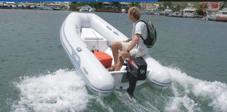
ے 2 **Overal Length** : 9'6"/ 2.90m **Number of Chambers** Maximum HP : 15hp / 11.2kw **Overal Beam Person Capacity** : 5 : 5'6"/ 1.68m Shaft Length : 15" / 38.1cm Inside Length Weight : 95lb / 43kg : 6'11"/ 2.11m RDC Design Category : C Inside Beam Weight with Bow Locker: 108lb/49kg : 2'6"/ 0.76m Recommended HP Tube Diameter : 17"/ 0.43m : 8hp / 6.0kw
