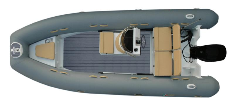
S ے S **Overal Length** : 18′/ 5.49m Number of Chambers : 5 Shaft Length : 25" / 63.5cm **Person Capacity** Gas Built in Tank : 32 Gal / 120 L **Overal Beam** : 7' 10"/ 2.40m : 12 RDC Design Category : C Inside Length : 895lb / 406kg : 14′8″/4.47m Weight
