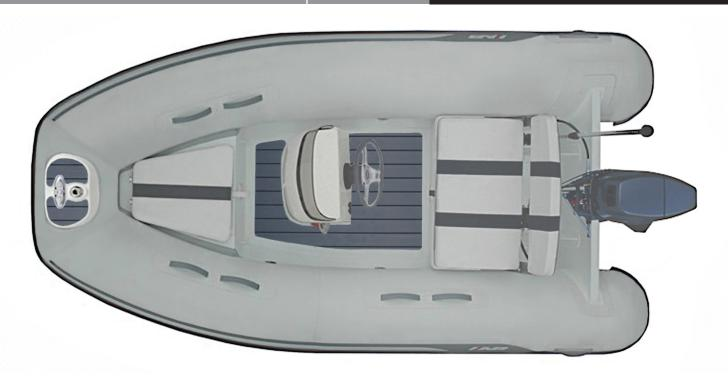
Overal Length : 10'6"/3.19m Number of Chambers : 3 Shaft Length **Overal Beam Person Capacity** RDC Design Category : C : 5'6"/ 1.68m Inside Length : 7'6"/2.30m Weight : 255lb / 116kg Recommended HP Inside Beam 2'8"/ 0.81m : 15hp / 11.2kw **Tube Diameter** : 17"/ 0.43m Maximum HP : 25hp / 18.7kw
