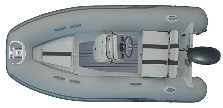
$\triangle$ S **Overal Length** Number of Chambers : 3 : 11'6"/3.50m **Overal Beam Person Capacity** : 5′7″/ 1.70m : 5 Inside Length : 8'6"/2.60m Weight : 284lb / 129kg Inside Beam : 2'8"/ 0.81m Recommended HP : 20hp / 14.9kw **Tube Diameter** Maximum HP : 17"/ 0.43m : 30hp / 22.4kw
