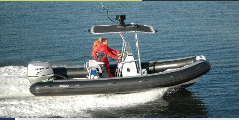
Overall Length : 19′/ 5.79m Number of Chambers : 5 Shaft Length : 25" / 63.5cm Gas Built in Tank Overall Beam : 8'4"/ 2.53m Person Capacity : 15 : 44 Gal / 167 L Inside Length : 15'2"/ 4.62m RDC Design Category: C Weight : 1157lb / 526kg Inside Beam : 4'1"/ 1.25m Recommended HP :115hp / 85.8kw
