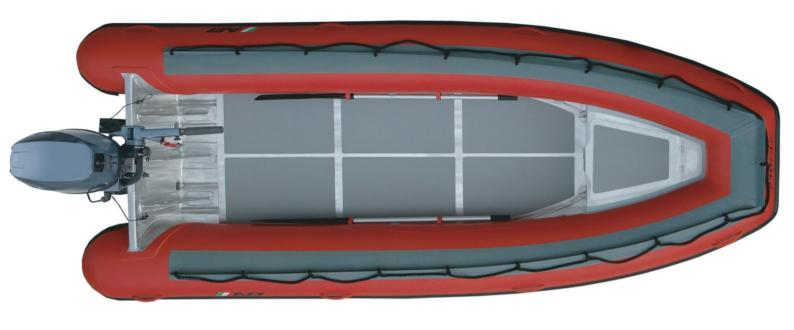
**Overal Length** Number of Chambers : 4 : 14'/ 4.27m Maximum HP : 50hp/37.3kw **Overal Beam** : 6'7"/ 2.00m **Person Capacity** : 8 Shaft Length : 20" / 50.8cm Inside Length 10′10″/3.30m Weight : 287lb/130kg RDC Design Category : C Inside Beam : 3'3"/ 0.99m Weight with Bow Locker: 305lb/138kg **Tube Diameter** : 19"/ 0.48m Recommended HP : 40hp /29.8kw
