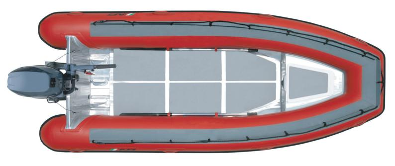
ے S Overal Length : 13'/ 3.96m Number of Chambers : 3 Maximum HP : 40hp / 29.8kw **Overal Beam Person Capacity** : 6'7"/ 2.00m **Shaft Length** : 20" / 50.8cm Inside Length : 9'10"/ 3.00m Weight : 256lb/116kg RDC Design Category : C Inside Beam : 3'3"/ 0.99m Weight with Bow Locker: 271lb/123kg Recommended HP Tube Diameter : 18"/ 0.46m : 30hp /22.4kw
