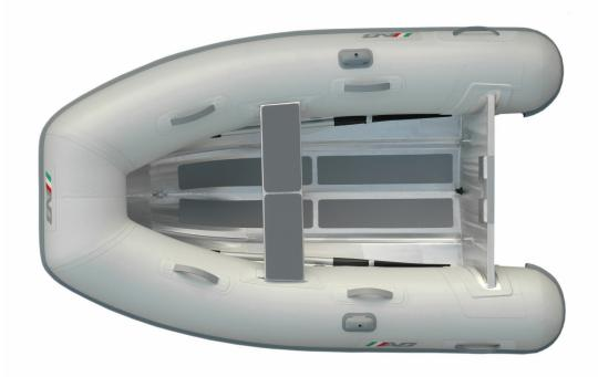
؎ S **Overal Length** : 7'10"/2.39m Number of Chambers : 2 Shaft Length : 15" / 38.1cm **Overal Beam** : 4'11"/ 1.50m **Person Capacity** RDC Design Category : C Weight Inside Length : 5'5"/ 1.65m : 66lb / 30kg Recommended HP Inside Beam 2'2"/ 0.66m : 3hp / 2.2kw **Tube Diameter** : 16"/ 0.41m Maximum HP : 4hp / 2.9kw
