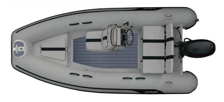
**Overal Length** : 13′/ 3.96m Number of Chambers : 3 Shaft Length : 20" / 50.8cm **Overal Beam Person Capacity** : 7 RDC Design Category : C : 6'7"/ 2.00m Inside Length : 9'10"/3.00m Weight : 372lb / 169kg Inside Beam Recommended HP : 3'3"/ 0.99m : 30hp / 22.4kw **Tube Diameter** : 18"/ 0.46m Maximum HP : 40hp / 29.8kw
