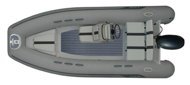
**Overal Length** : 14′/ 4.27m Number of Chambers : 4 Shaft Length **Overal Beam Person Capacity** RDC Design Category : C : 6'7"/ 2.00m : 8 : 10′10″/3.30m Inside Length Weight : 392lb / 178kg Inside Beam Recommended HP : 3'3"/ 0.99m : 40hp / 29.8kw
