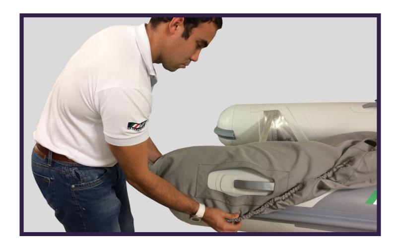
Start from one of the dinghy cones adjusting the fabric below the rub rail.
