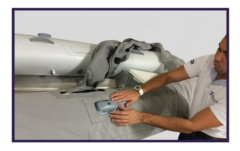
Continue towards the bow adjusting the holes with the handles, oarlock bases & seat retainers.
